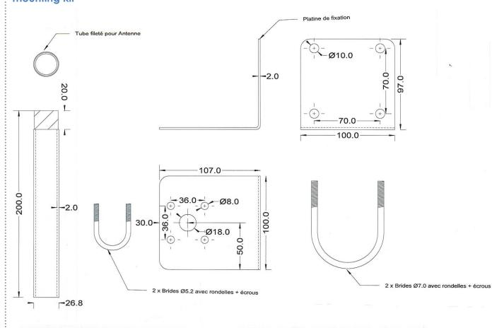
GPS antenna installation using the mechanical Kit
