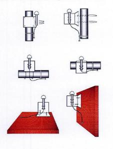
Where to install the GPS antenna
