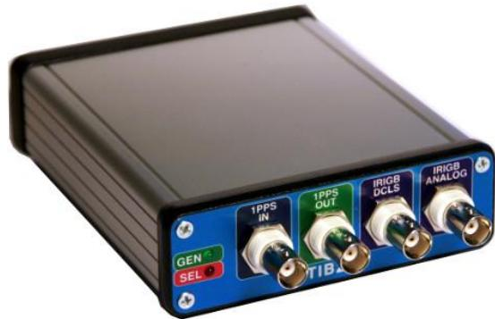
To use the TIB, simply connect it to an USB port of a PC or an USB hub. The TIB is powered through the USB connection and don't require an external power supply.
